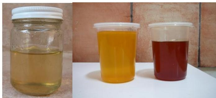
Figure 1. Color variation of the samples, from water white to light amber.
